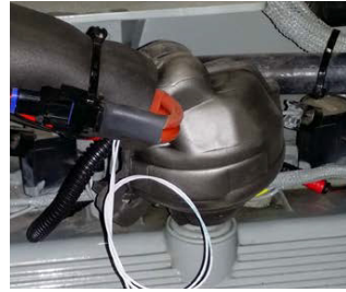
IntelliThaw Heating Jacket on a PCV Filter in a diesel engine
