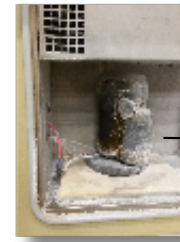
Kapton Heater 14 VDC 13.6 Amps
