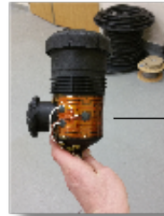
Kapton Heater 14 VDC 13.6 Amps
